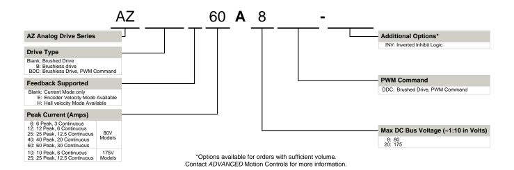
ADVANCED Motion Controls AZ series of servo drives are available in many configurations. Note that not all possible part number combinations are offered as standard drives. All models listed in the selection tables of the website are readily available, standard product offerings.
