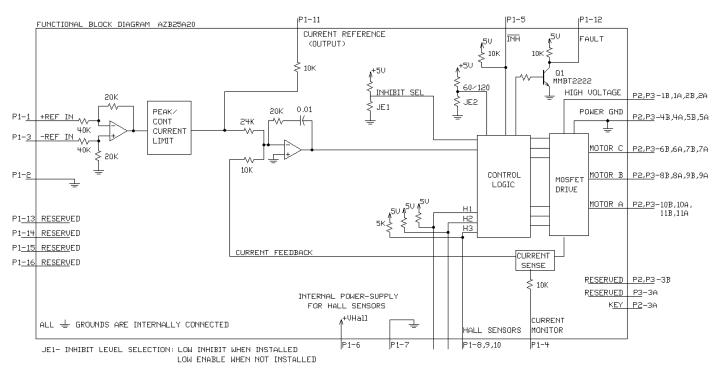
JE2- PHASING: 120 DEGREE WHEN INSTALLED, 60 DEGREE WHEN NOT INSTALLED
