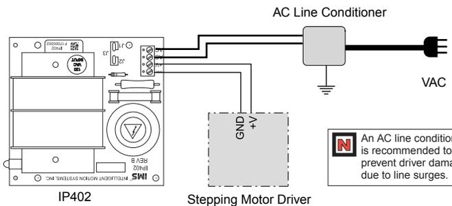
**N** An AC line conditioner is recommended to prevent driver damage due to line surges.
